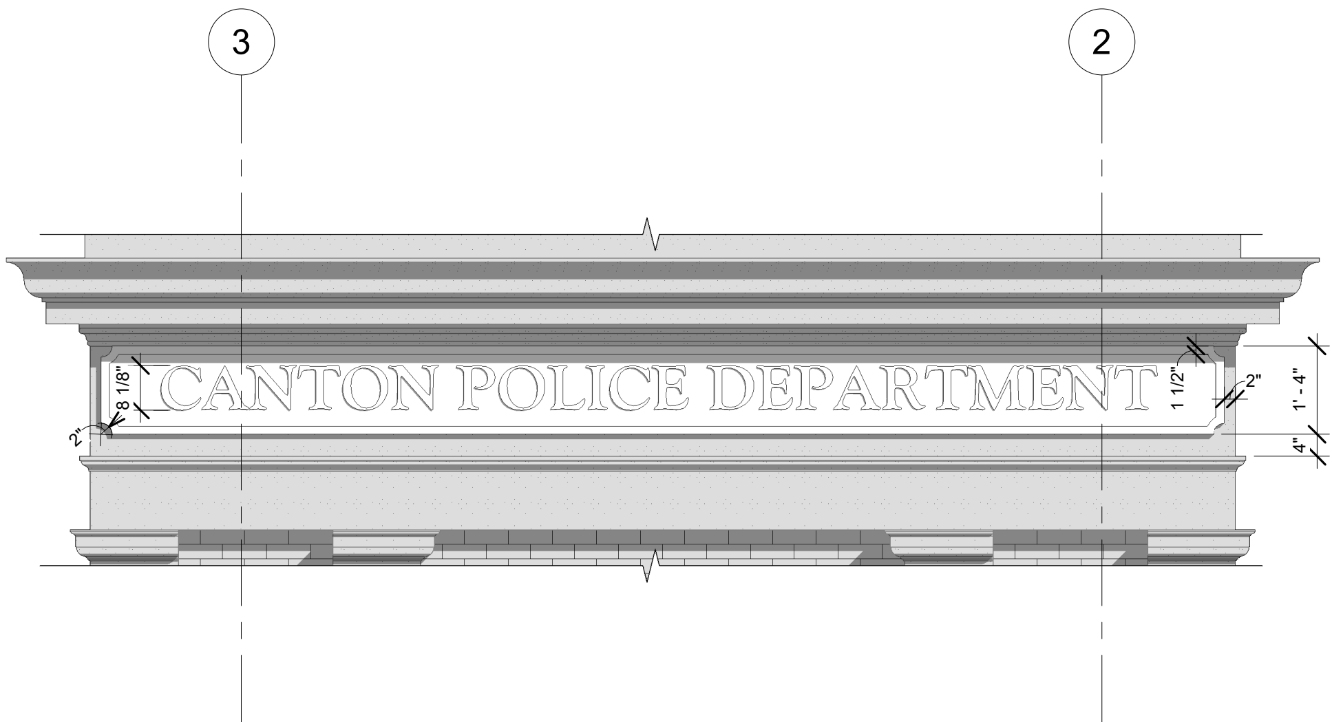
CS-1 3" = 1'-0" *PROFILE & SILL TO MATCH EXISTING, V.I.F.
